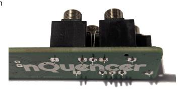
4. Solder one pin of the button while pushing the button down, then check you are happy with the position of the button and it can be pushed smoothly. If you want to adjust it, reflow the pin you have just soldered while repositioning the button. When you are happy with the position, solder the other pins of the button and then solder the five jack sockets.
