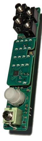
Without soldering anything yet, place the green socket and four black sockets on the main PCB. Pairs of black sockets share a hole on the PCB for their ground pins.
