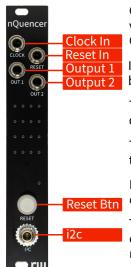
Connect nQuencer to your 16n faderbank via i2c, give it a Clock and it will output CV (Output 1) and a Gate (Output 2).
